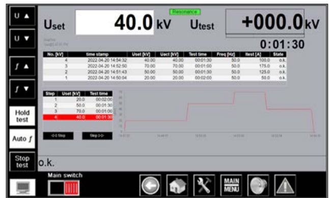
Figure 5: Data display during an automatic test sequence
