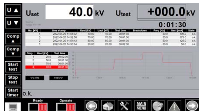
Figure 7: Data display during an automatic test sequence
