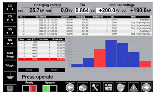
Figure 18: Data display during an automatic test sequence
