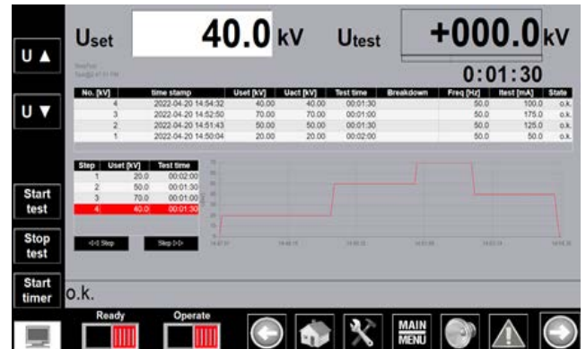
Figure 20: Data display during an automatic test sequence
